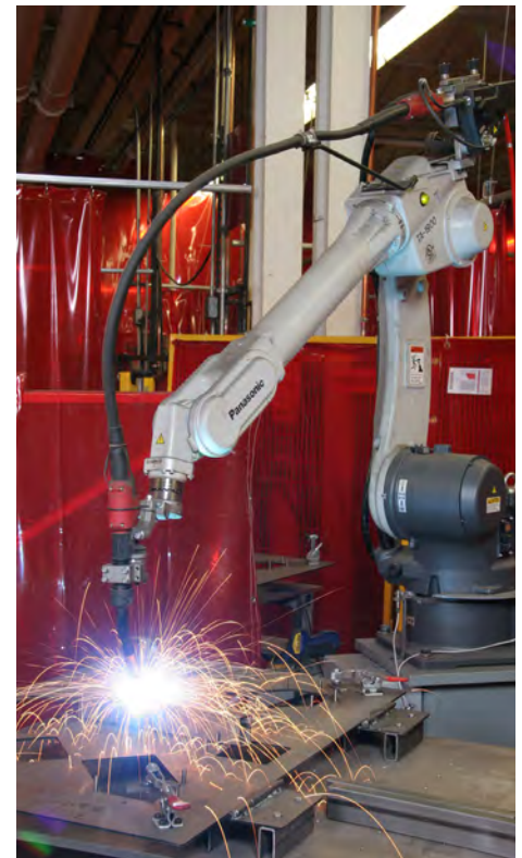
One of two newly acquired robotic mig welders allow for high speed and high-quality output.
