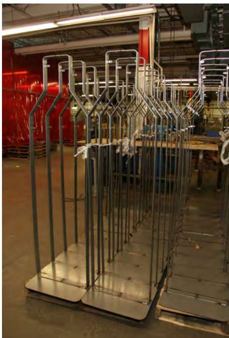
These display components for a liquor display await their next operation: powder coating.
